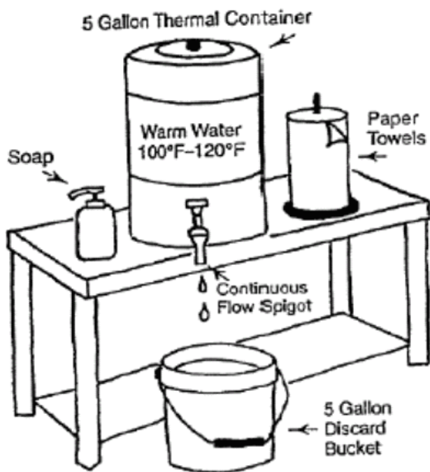
Proper Hand Wash Station
